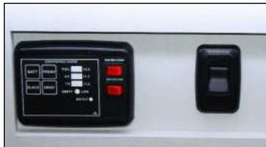
Centralized Monitor/Control Center
