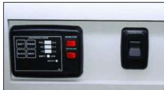
Centralized Monitor/Control Center
