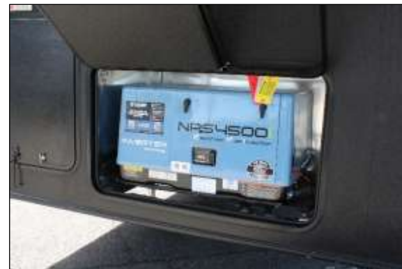
4.5 KW Yamaha Generator
