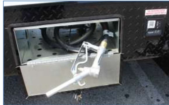
40-Gallon Fuel Station
