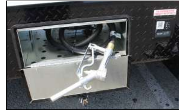
40-Gallon Fuel Station
