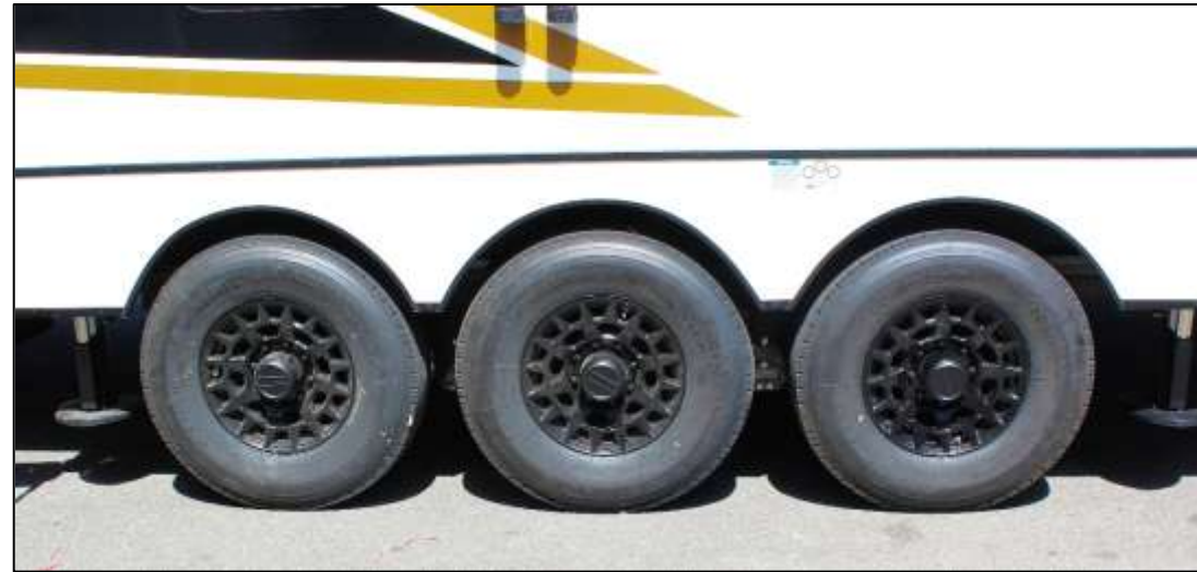
7000 Lb. Triple Axles w/16" Wheels & LR G Tires
