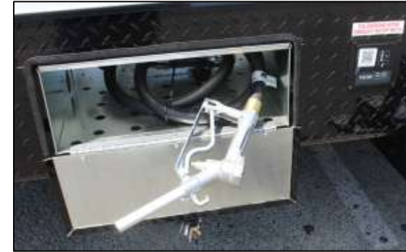
40-Gallon Fuel Station
