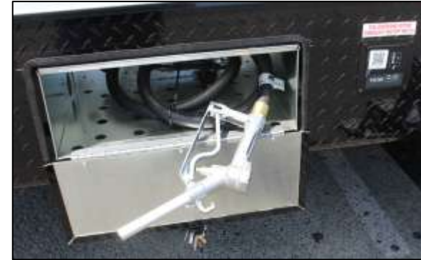
40-Gallon Fuel Station
