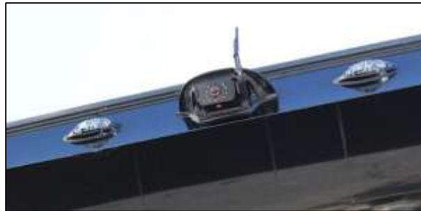
Patented Spoiler w/Wireless Backup Camera
