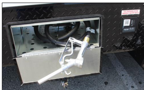
40-Gallon Fuel Station
