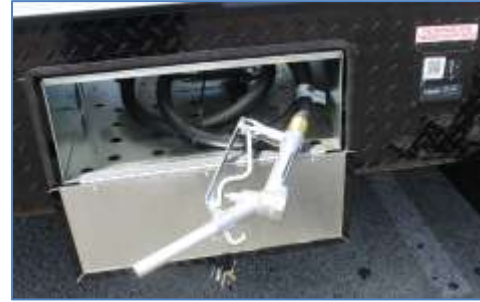
40-Gallon Fuel Station
