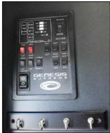
Central Monitor/Control Panel
