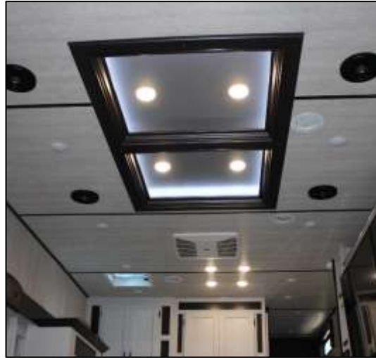
Coffered Ceiling Panel w/LED & Accent Lights
