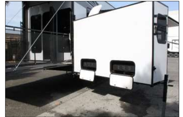
Cooktop Vent Fans w/Exterior Vents Open
