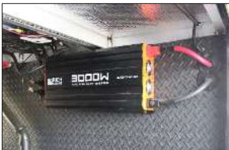
Optional 3000-Watt Inverter/Electrical Accessory Controls in Forward Compartment
