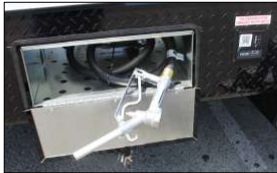
40-Gallon Fuel Station
