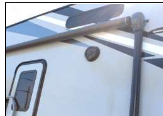
Powered Awning w/LED Strip
