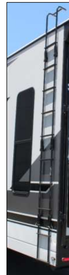
Exterior Folding Ladder & Walk-On Roof
