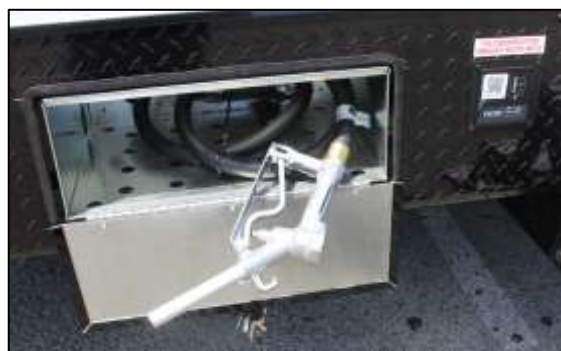
40-Gallon Fuel Station
