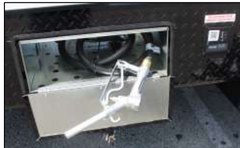
40-Gallon Fuel Station
