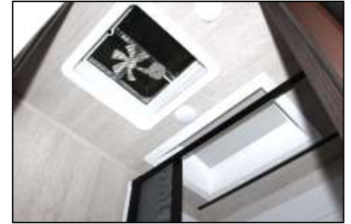
Lavy Overhead Vent & Skylight Over Shower
