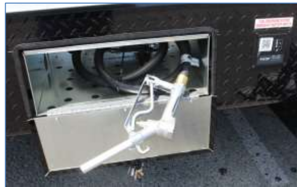
40-Gallon Fuel Station
