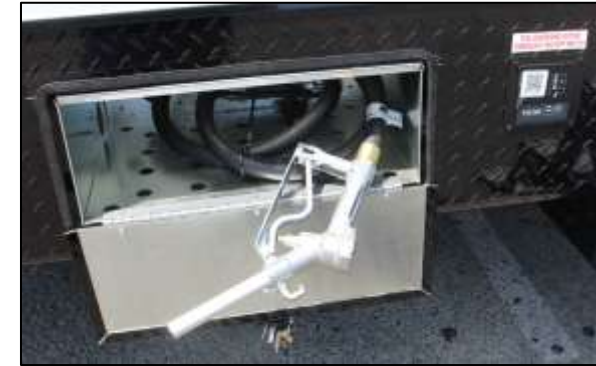
40-Gallon Fuel Station
