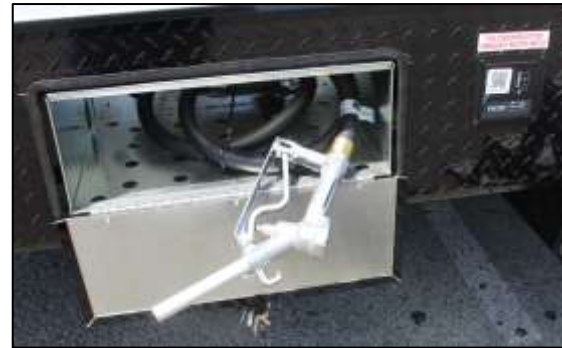
40-Gallon Fuel Station
