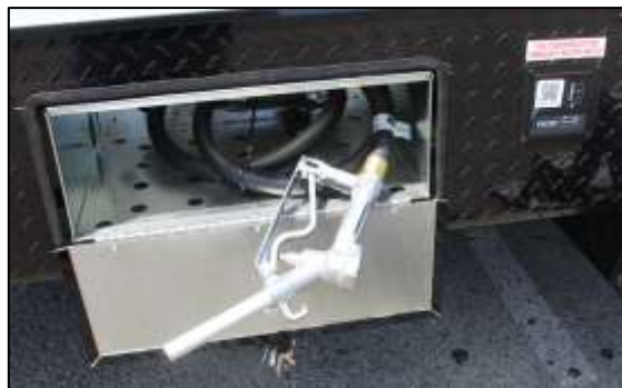
40-Gallon Fuel Station
