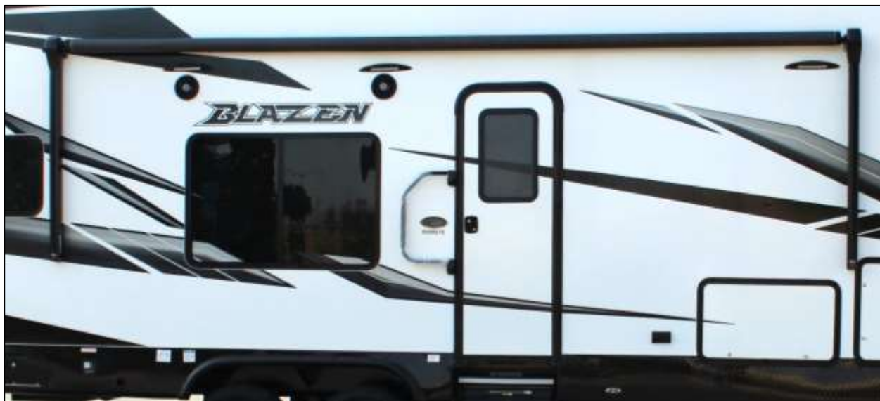
Power Awning w/LED Light Strip, Radius Glass Entry Door w/Window, Exterior Speakers, Fold-Away Entry Handle.
