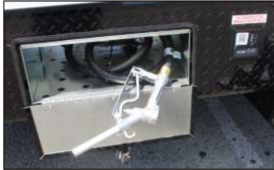
40-Gallon Fuel Station
