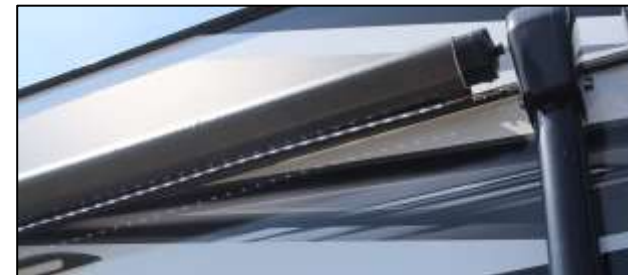
Powered Awning w/LED Strip
