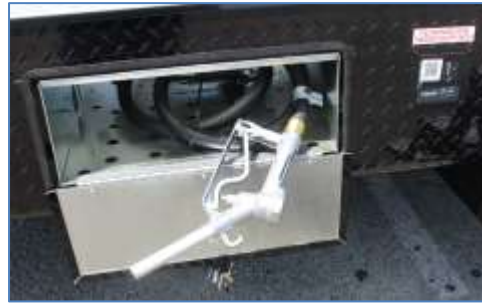
40-Gallon Fuel Station
