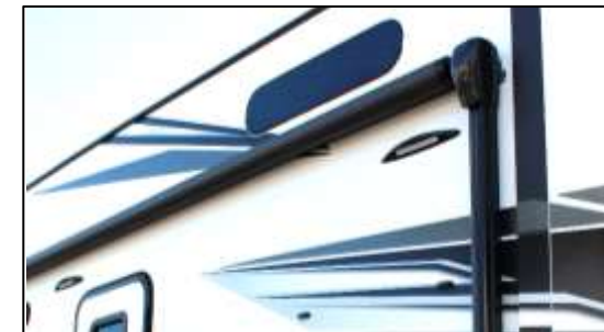
Powered Awning w/LED Strip
