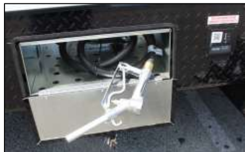
40-Gallon Fuel Station
