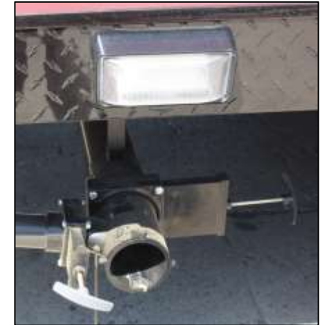
Light @ Drain Valves
