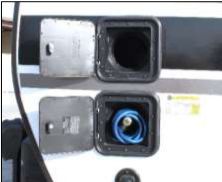
Sewer Hose Storage & Water Hose Sprayer
