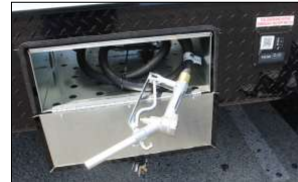
40-Gallon Fuel Station
