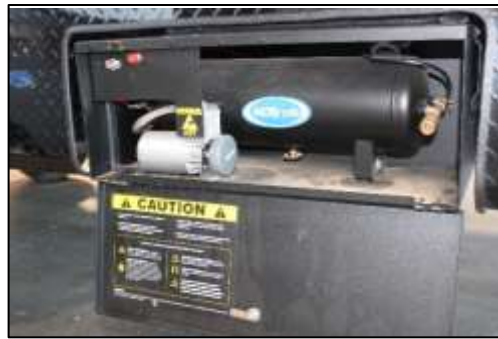
On-Board Air Compressor
