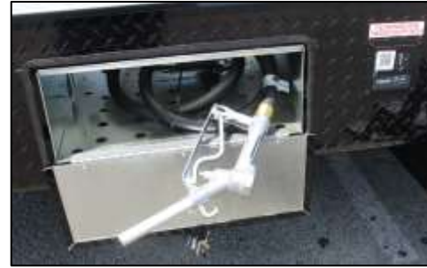
40-Gallon Fuel Station
