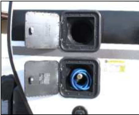
Sewer Hose Storage & Water Hose Sprayer
