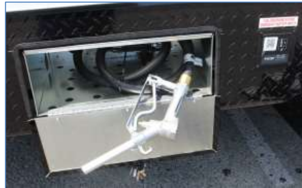
40-Gallon Fuel Station
