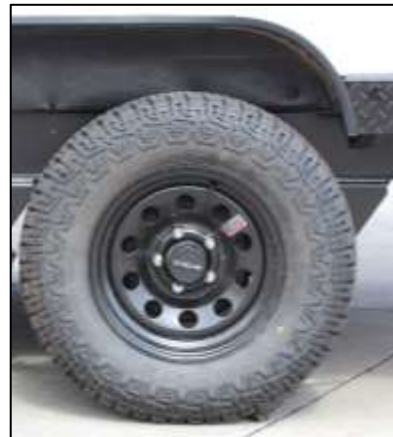
14" Aluminum Wheels w/Load Range D Tires
