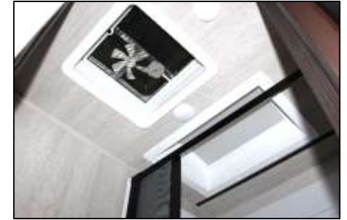
Lavy Overhead Vent & Skylight Over Shower
