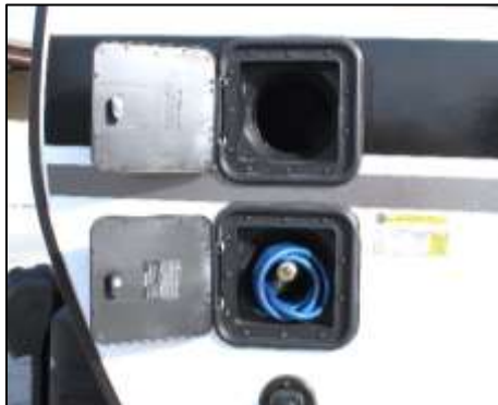
Sewer Hose Storage & Water Hose Sprayer
