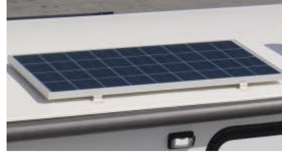
190-Watt Solar Panel & Controller Panel – Operates 12V Refer
