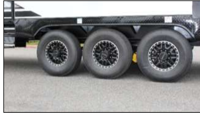
7000 Lb. Triple Axles w/16\" Wheels & LR G Tires
