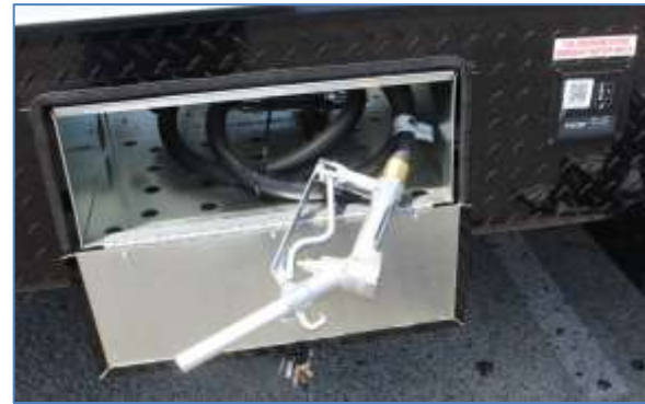
40-Gallon Fuel Station
