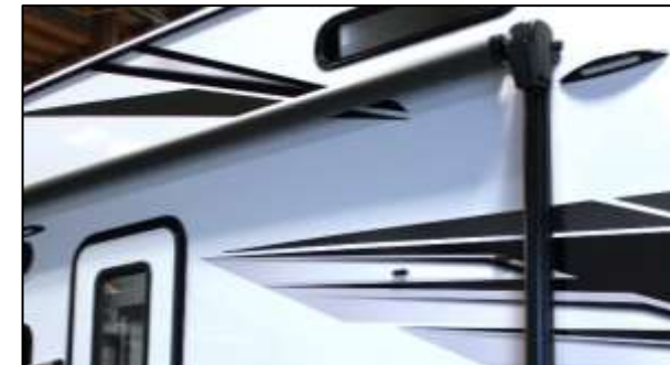
Powered Awning w/LED Strip
