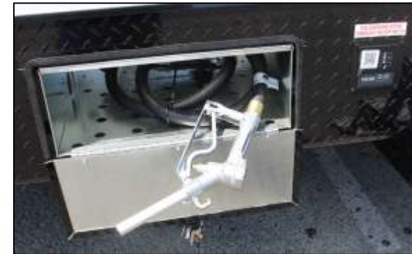
40-Gallon Fuel Station
