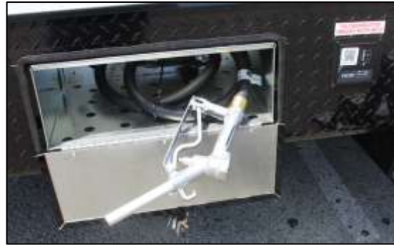
40-Gallon Fuel Station
