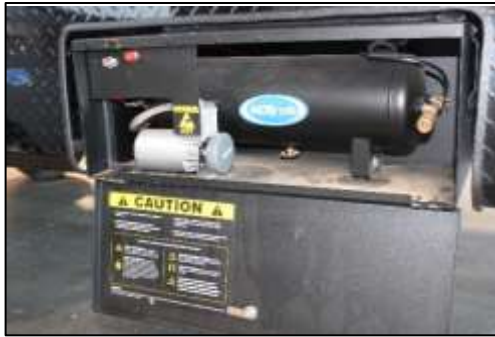
On-Board Air Compressor
