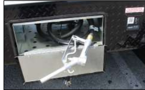
40-Gallon Fuel Station
