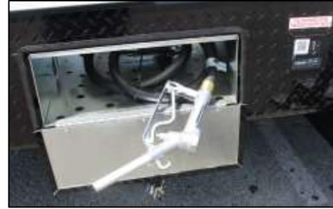
40-Gallon Fuel Station
