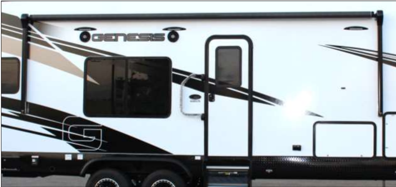
Power Awning w/LED Light Strip, Radius Glass Entry Door w/Window, Exterior Speakers, Fold-Away Entry Handle.
