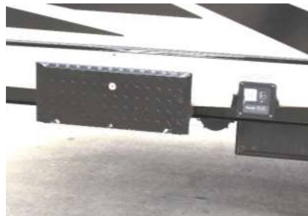
40-Gallon Fuel Station
