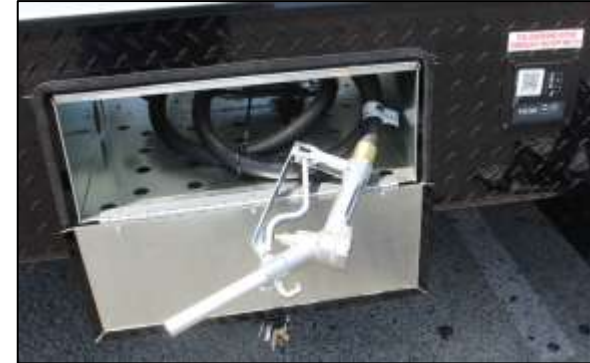
40-Gallon Fuel Station
