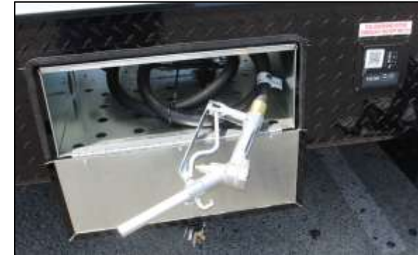
40-Gallon Fuel Station
