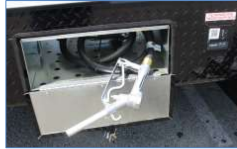
40-Gallon Fuel Station
