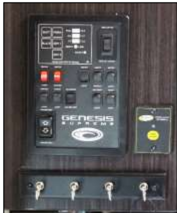
Central Monitor/Control Panel
