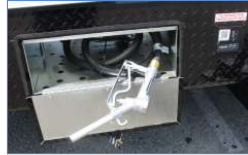
40-Gallon Fuel Station
