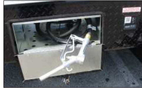
40-Gallon Fuel Station
